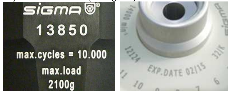
Fig. 5.9: Different service life – engraving on the bucket/rotor
