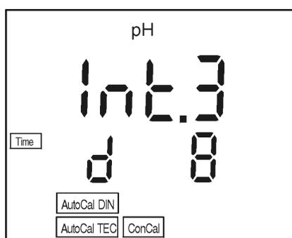
8 Set up the required time interval by pressing **<▲>** **<▼>**.
