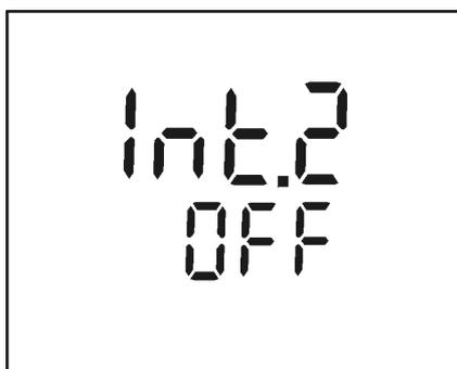
3 Press **<▲>** **<▼>** to set up the required time interval between storage processes.
