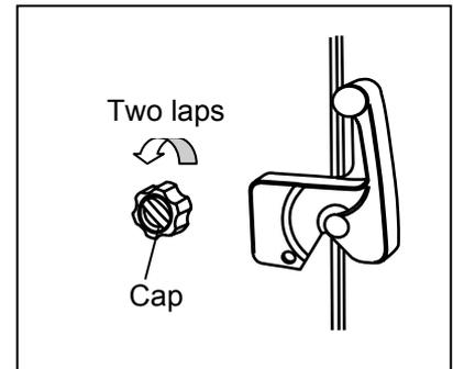
A door may not open in the above method when there are frost and ice in the air intake port. In that case, open a cap, and investigate the matter whether there is no frost inside the air intake port. Remove frost inside the air intake port by " Stick for air intake port cleaning " of the accessories when there is frost. Clean a air intake port every month even when there is no frost inside the air intake port. Refer to page 37.
