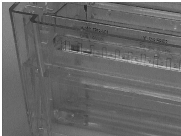
Fig. 4. Outlined sample wells and sample loading guides take the guesswork out of samples loading.
